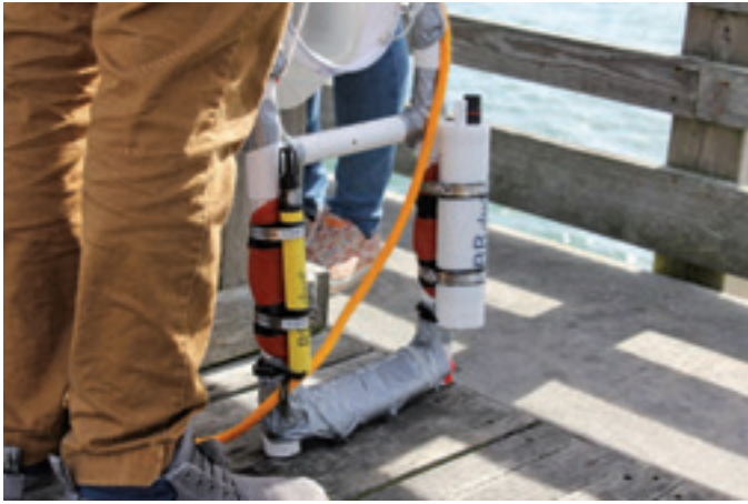
RBR duet T.D and RBR duo T.DO mounted on the plankton net tow frame, christen "the Bagel" by the Phyto-Finders.
