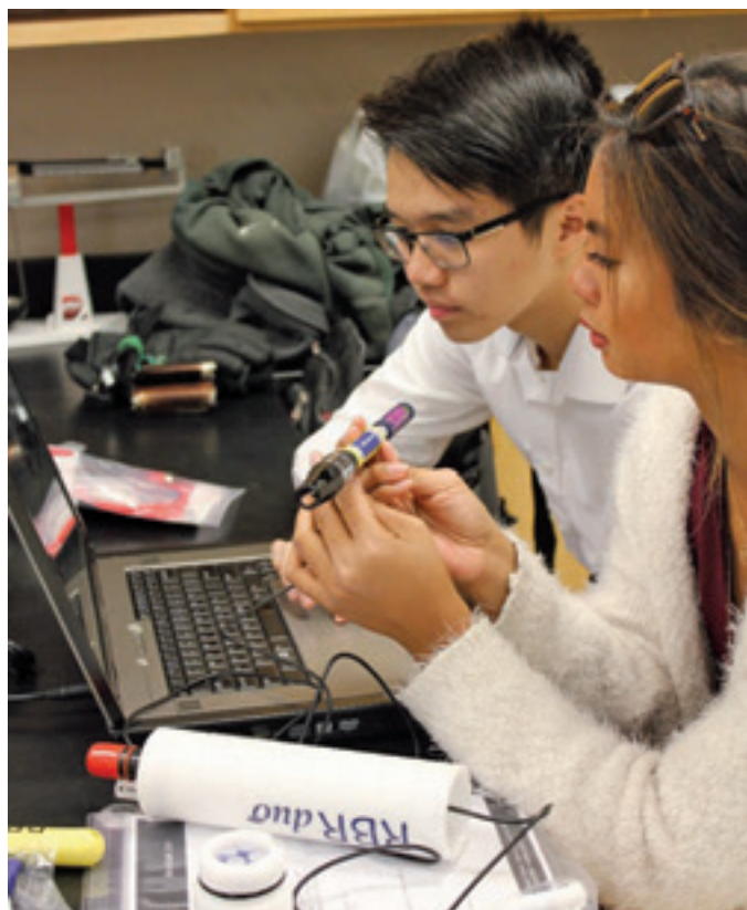
Seniors Ben Tran and Julia Bachman program the RBR loggers and run a bench top deployment.
