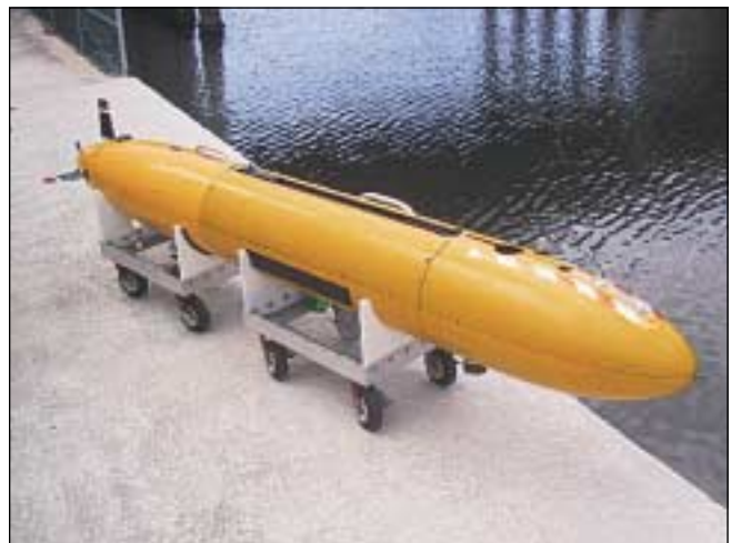
Fig. 1: Ocean Explorer UUV operated by the NATO SACLANT Undersea Research Center. This UUV is being equipped with an 8-16 kHz low frequency SAS for buried mine detection, which will be tested at sea in October 2002. The SAS receiver array features 4 rows of 16 elements spaced at 6.25 cm. Both the UUV and the SAS were manufactured by Florida Atlantic University.
