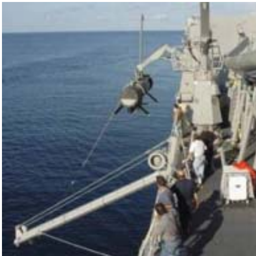
Remote Minehunting Vehicle is lowered to the water by a unique dual-arm davit.
