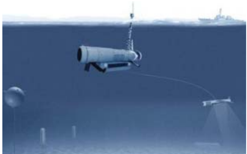
Remote Minehunting Vehicle towing Variable Depth Sonar
